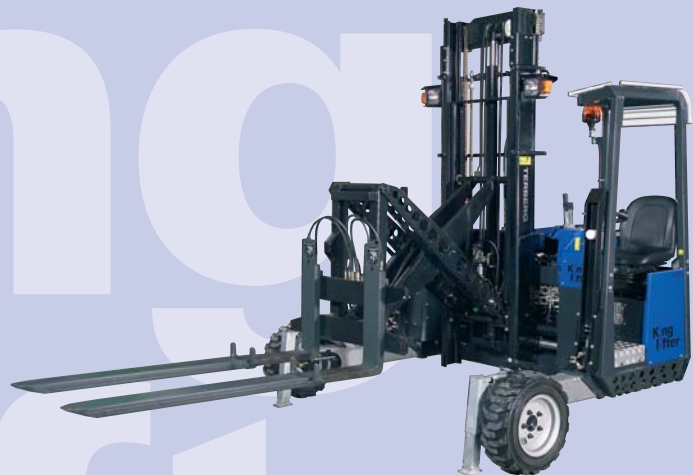
The 4-way steering system transforms the truck mounted forklift into an advanced side loader.
