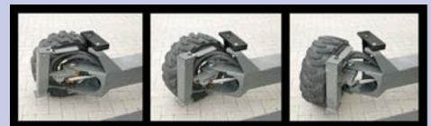
The 4-way steering system transforms the truck mounted forklift into an advanced side loader.
